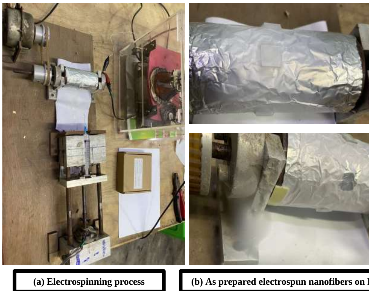
Figure 3(a, b) Preparation of Zinc Stannate nanofiber photoanodes
