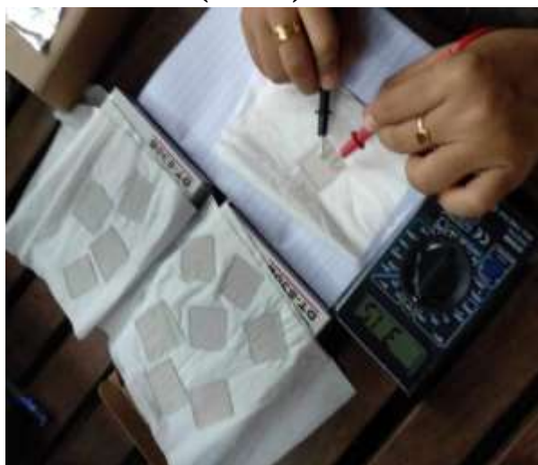
Figure 2 Cleaning process of FTO Glasses and checking conductive side
